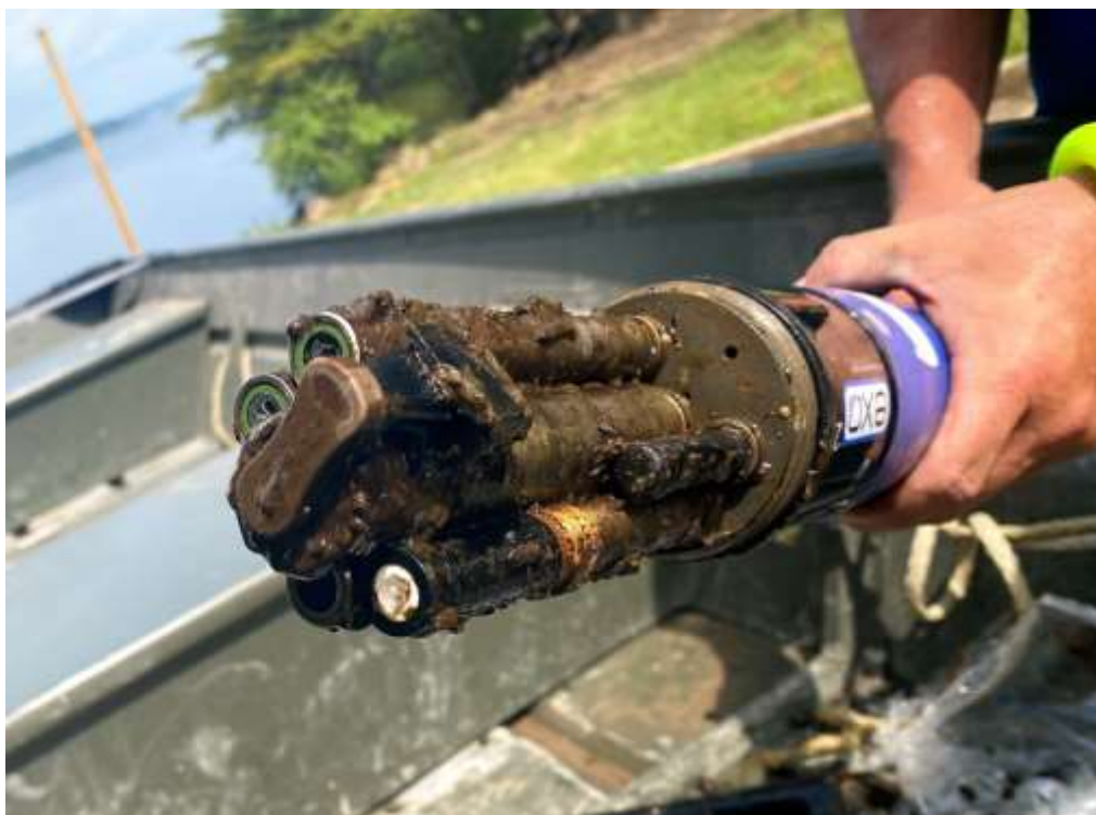
Figure 35: Water Quality Sonde After Eight-Week Deployment at NETMWD Intake
