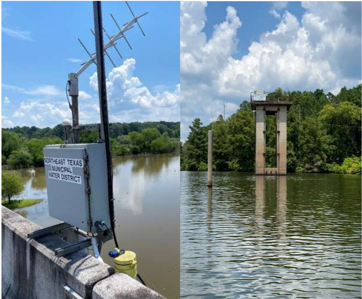
Figure 33: US 259 (left) and NETMWD Intake (right) Continuous Water Quality Monitoring Stations
