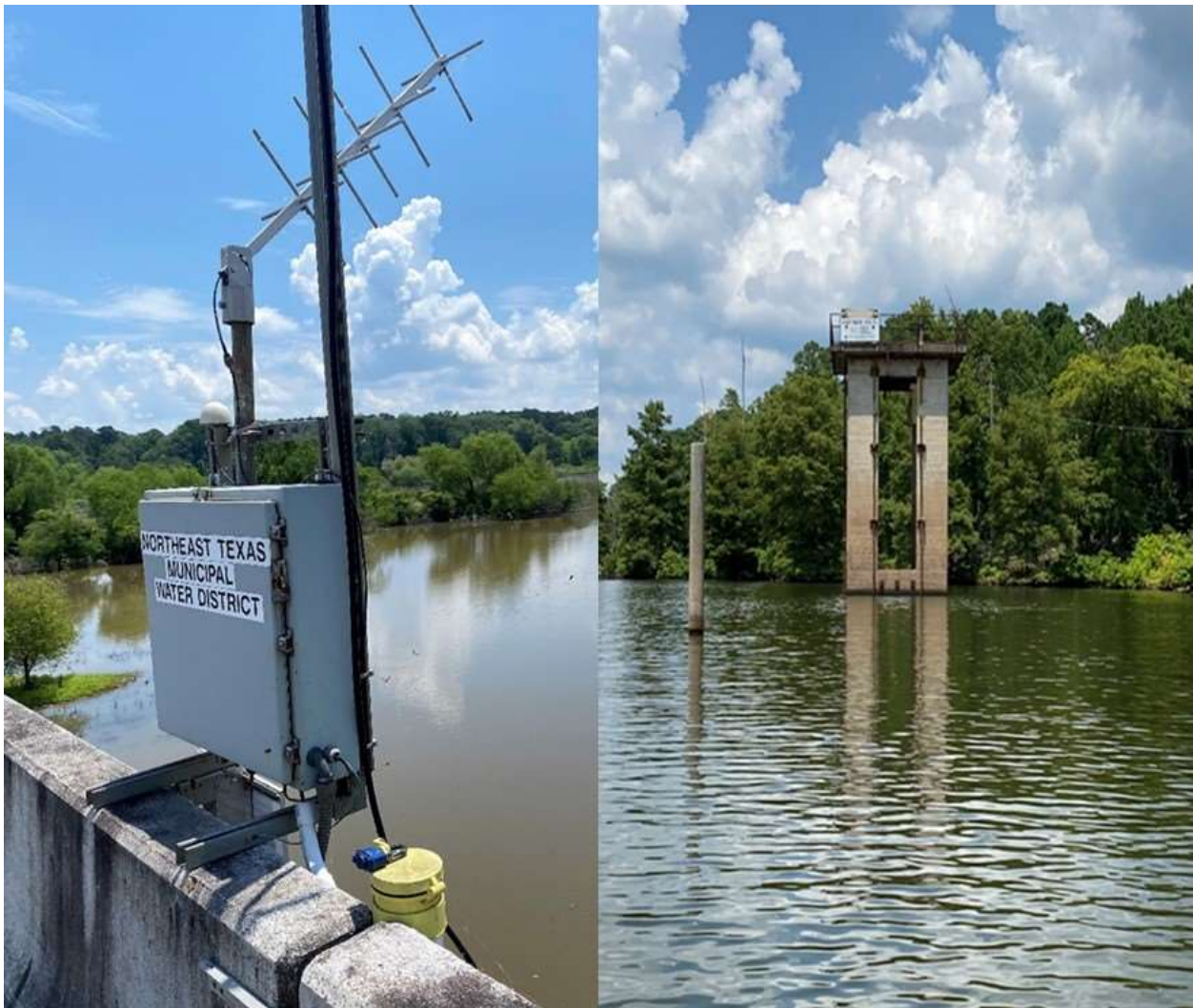
Figure 53: Lake O' the Pines continuous water quality monitoring stations; US 259 station (left), NETMWD intake (right)
