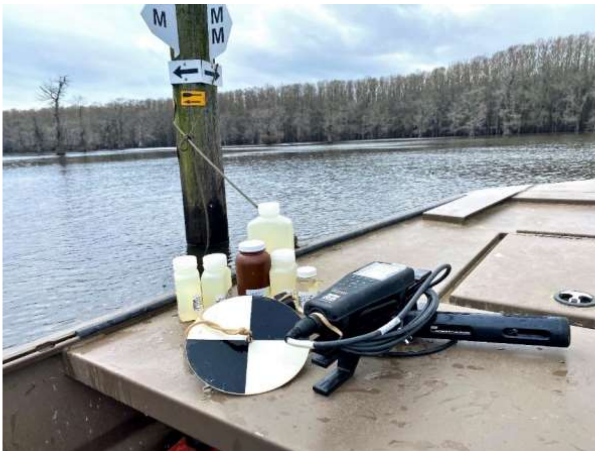
Figure 7: Sample bottles and instruments used to measure field parameters
